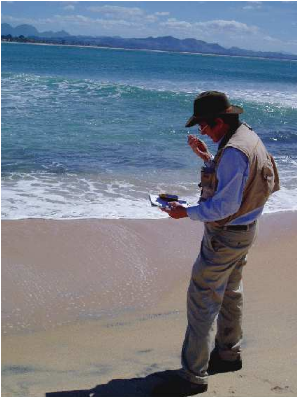
Figure 2. Example of GPS measurement, allowing precise surveying of the site (in this case Site 6, on Ampandrozonana Beach in Sambava), and in addition, a computation of the inundation parameter, by differential GPS surveying.
