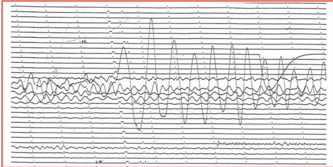
Figure 4. Example or record used in the PDFM inversion. This is the Rayleigh wave R_1 recorded on the vertical Benioff 1-90 instrument at Pasadena.
